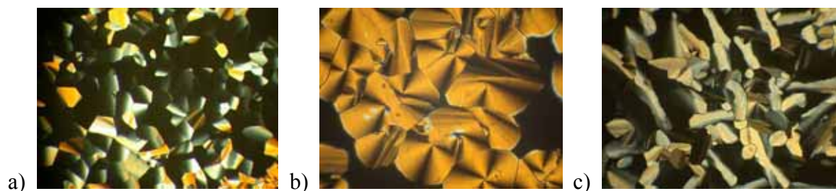
Figure 3.10. Textures of the columnar phases of: (a) compound Na6.16/3 at 87 °C; (b) compound Na6.16/4 at 73 °C; (c) compound Na6.16/6 at 78 °C.
