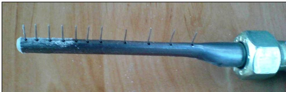
Figure 3.4 Spacing arrangements for the thermoelements
