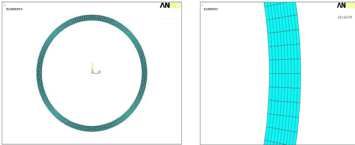
Figure 2.3a and 2.3b Numerical modeling grid for the Rotary Kiln
