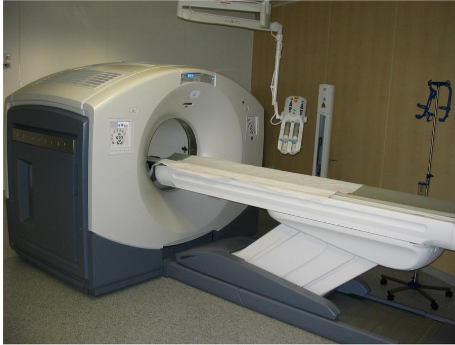
Figure 10: A PET/CT scanner. The frontal part of the gantry features a CT scanner, while the rear part contains a PET scanner.
