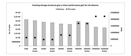
Figure 6.15: Performance comparison of different DSM based schemes in ECOS with a primary key based search criteria.
