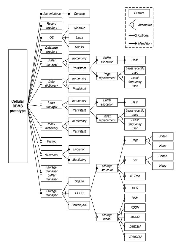
Figure 5.3: The Cellular DBMS prototype feature model.
