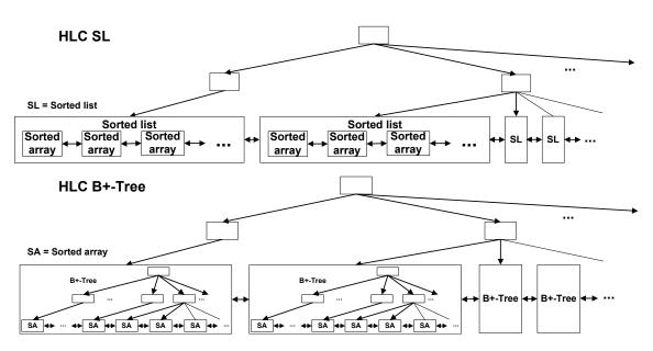
Figure 4.3: HLC SL and HLC B+-Tree storage structures in the Cellular DBMS prototype.
