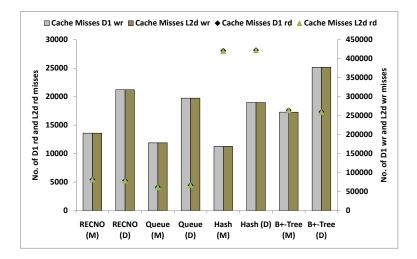
Figure 6.3: Micro benchmark results using the Berkeley DB: Minimal configurations cause less data cache write misses.
