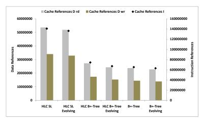
Figure 6.10: Evolving storage structures generate less cache references.
