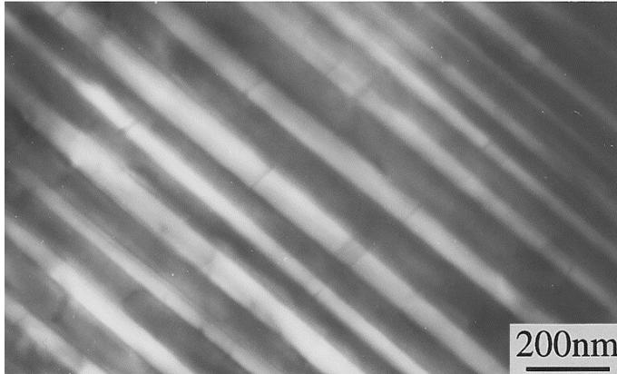
Figure 2.3: Electron micrographs of Ti-62.5at.%Al alloy annealed at 930°C, taken from [130]
