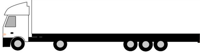
Figure II.3: Semi-Trailer Truck with Tridem Trailer Axle
