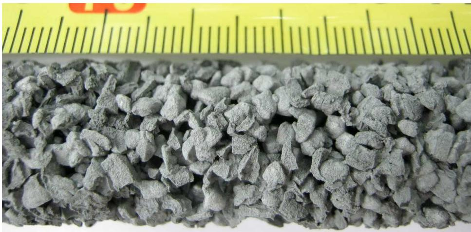
(b) Detail view of the CWGSR fixed bed. Visible is the high porosity of granular the material.
