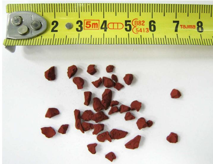
Figure 2.2.: Pellets made from  $\text{Fe}_2\text{O}_3$  and sodium silicate after preparation.
