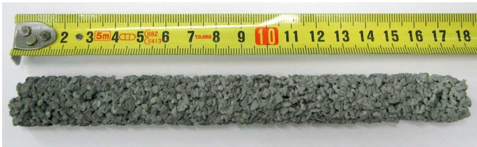
(a) Slightly fused part of the fixed bed. The missing length disintegrated to its constituent pellets upon removal from the CWGSR tube.
