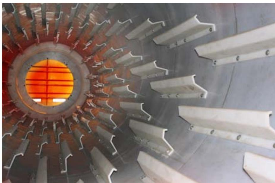
Figure 1.7: Cross sectional view of an industrial rotary dryer showing flights (Feeco, Inc., Wisconsin, USA).
