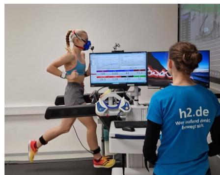
**Figure 3.** Laboratory setup with motorized treadmill, spirometry, subject wearing the OWN footwear condition, and researcher supervising the trial.
