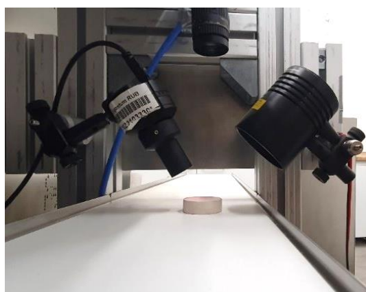
Figure 1: Measurement setup over a conveyor belt (middle, white). On the left, the NIRS Viavi 1700 ES measures NIR reflection of the light of the tungsten halogen lamp (right) from a sample. Mounted on top is a camera, which triggers a measurement when a sample particle is detected.
