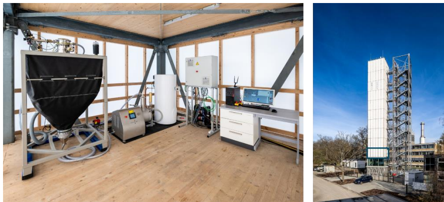
Figure 2. Thermochemical energy storage based on quicklime in the D1244 at the University of Stuttgart.
