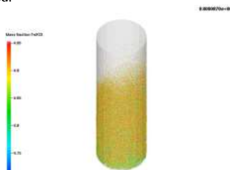
Figure 2. Simulation of a bubbling bed iron reduction reactor
