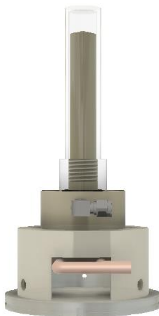
Figure 2: 3D-rendered illustration of the in-situ freeze-drying stage [3]
