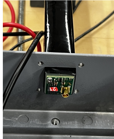
(b) Photo of assembled PCB glued onto a scintillator bar on a test stand.
