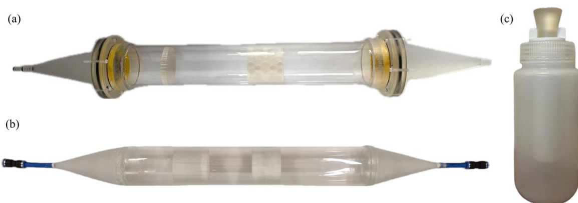
Figure 1: Pictures of water flow (a), gas flow (b) and temperature setup (c). Note here the inner white tube filled initially with hot water is inserted in the plastic bottle filled with water at room temperature.
