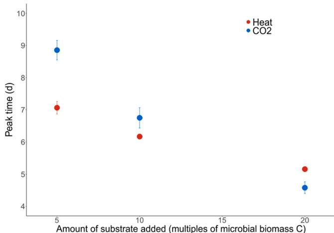
**Fig. 4.** The time of peak in heat and CO<sub>2</sub> curves (different colors) for different amounts of cellulose added based on soil MBC at 20 °C and 23 % gravimetric soil moisture. Bars represent 95% confidence intervals. (For interpretation of the references to color in this figure legend, the reader is referred to the Web version of this article.)
