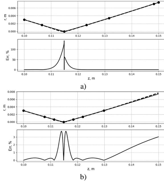
Figure 4: Illustration of solving interpolation task (a) and combined interpolation-extrapolation task (b) for EB boundary trajectory with simulation task parameters:  $U_{ac} = 25$  kV,  $I_b = 0.6$  A, and  $r_{b0} = 3$  mm.
