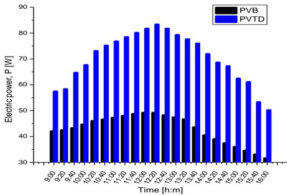
Figure 8: Time dependence of PVB and PVTD electric powers.
