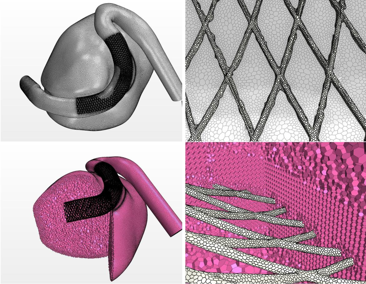
Figure 7.5: Mesh resolution of the analyzed case at different locations
