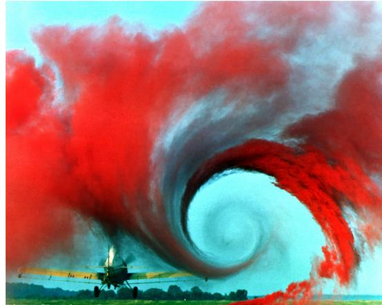
Figure 4.8: Wingtip vortex generated by an airplane; Source: NASA; Photo ID: EL-1996-00130; Alternate ID: L90-5919
