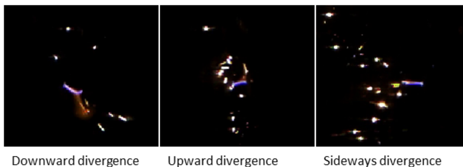
Figure 6.15: Effect of the electrical arc shape on the particle divergence direction
