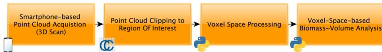
FIGURE 2 Workflow description: After point cloud acquisition via smartphone, point clouds were clipped, voxel space was processed, and finally, relationships between resulting voxel volumes and the harvested biomass were evaluated.
