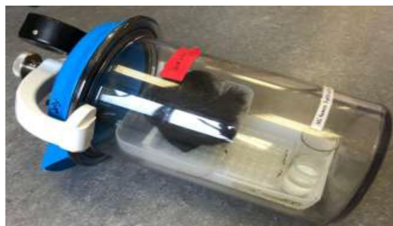
Figure S 1: Hypoxic chamber for the investigation on M. abscessus LOPs in an anaerobic pot, commonly used in culturing anaerobic bacteria on solid medium. Due to the round shape, the set up needs to be performed in a lying position and vials with indicator (top, right side) and carbonate solution (bottom, right side) are placed in a tray to avoid tipping over. The activated iron wool is placed in an extra tray (to prevent contamination by oxidation products) on top of the microtiter plates. Due to the unfavourable shape, this set up takes up a lot of space, but it can be used if no other airtight boxes are available.
