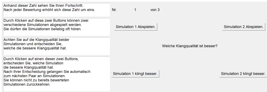
Figure 4.1: Screenshot of the graphical user interface (GUI) for pairwise comparison during training task with short instructions. On the left, all the components of the GUI are explained. On the right, two cochlear implant (CI) simulations to be compared can be listened to via two buttons. The simulation with the better sound quality is selected via one of the two other buttons below.
