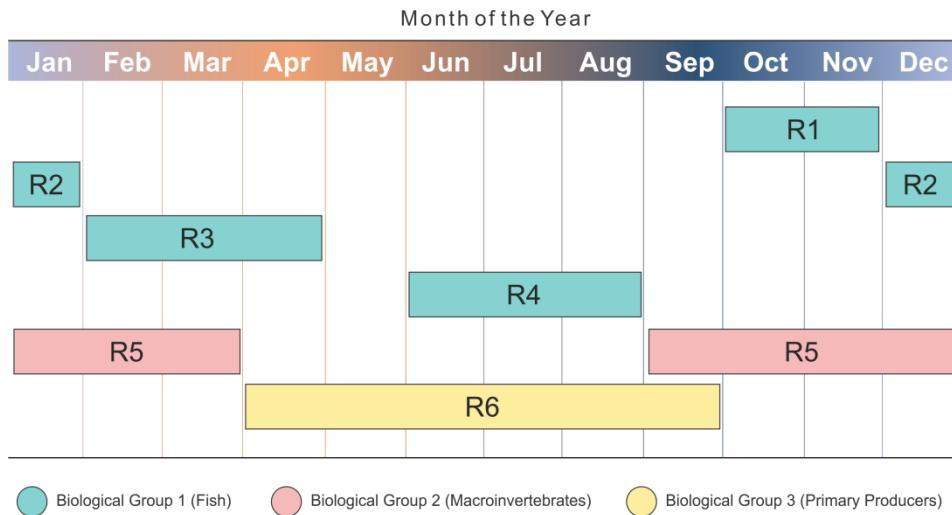
Figure 8 **Annual distributions of e-flow requirements defined for the Pas River.** Each requirement has been translated into the ecological objectives within the optimization model for water diversion.
