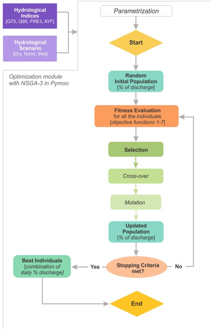
Figure 5 **Optimization problem structure employed to the Pas River.** The main box shows the module structure of the Non-Sorted Genetic Algorithm-3 (NSGA-3) in Pymoo – multi-objective optimization in Python. Two external modules, Hydrological Scenario and Hydrological Indices, calculate the hydrological scenarios to be inputted into the Pymoo module and the hydrological variables, respectively.
