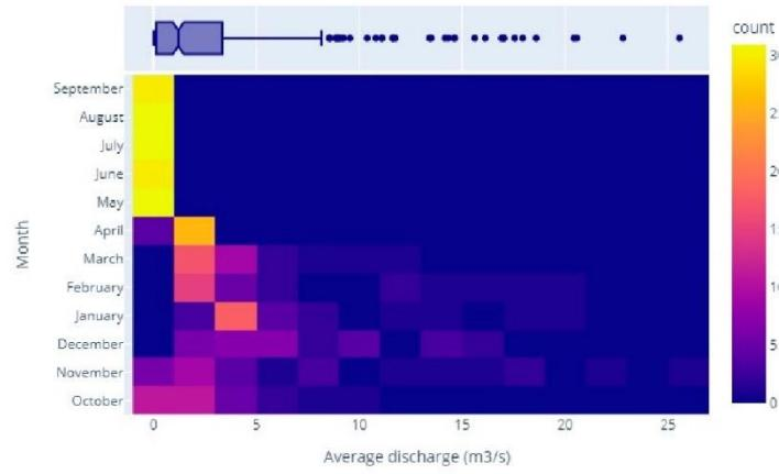
**Figure S10.** Heatmap showing the average optimized discharge (in m³/s) value (on the x-axis) for each month (on the y-axis) for the 2041 BGIN\_CC scenario. On the right-hand side of the box a colour-based classification of the frequency of appearance of each value range; on top of the box a regular box-plot shows the yearly quartiles, extremes and outliers.
