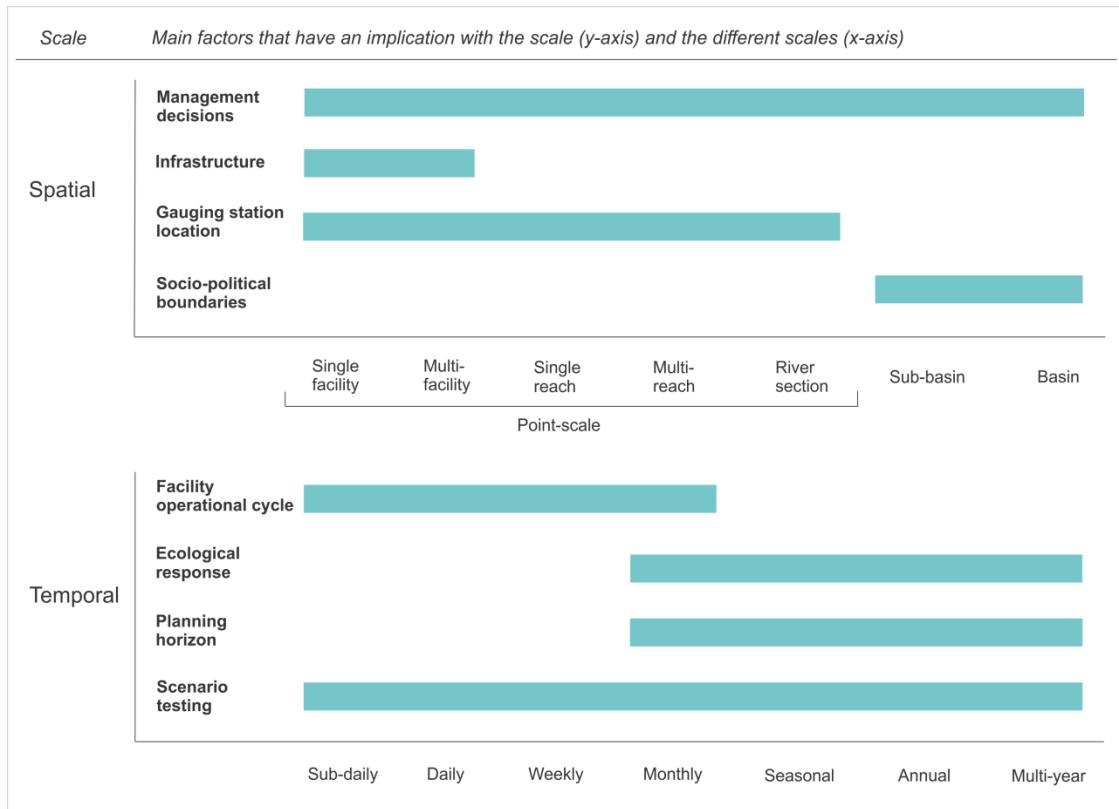
**Figure 3 Temporal and spatial scales that define water management optimization problems.** This figure is based on the results of our analysis. It illustrates the different spatial and temporal scales in relation to certain factors which challenge optimization procedure development by means of decision and option selection complexity, and definition of the resulting system boundaries.
