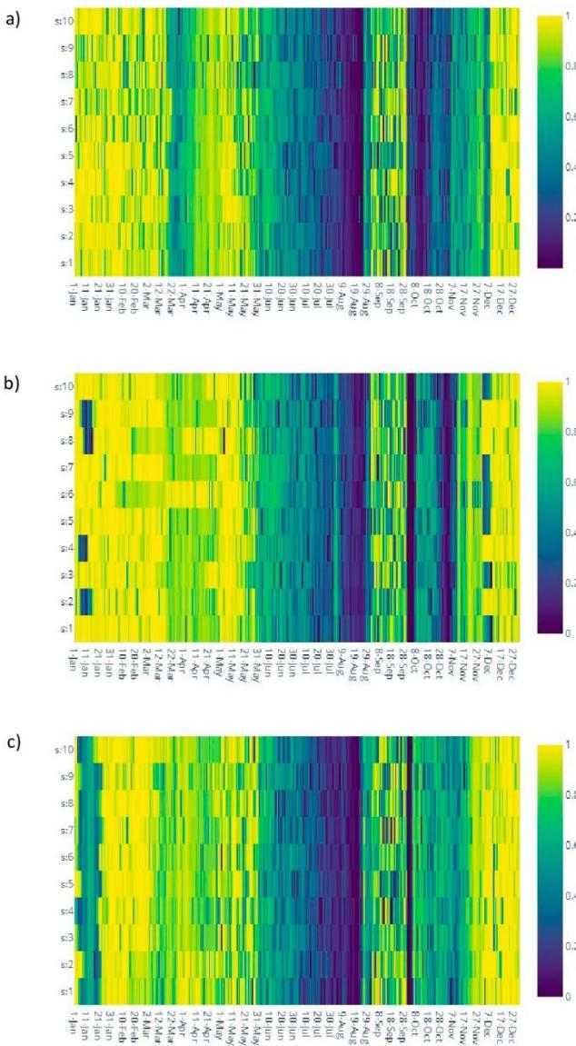
**Figure S2.** Combination of the average daily diversion percentages with respect to the natural discharge normalized to 0-1 range for each single run of the model ('s1-s10') under the same scenario. Yellow (1) tiles correspond with the highest diversion percentage, whereas blue (0) tiles correspond with the lowest optimal diversion. **Results for DP1** under dry (a), normal (b) and wet (c) scenarios.
