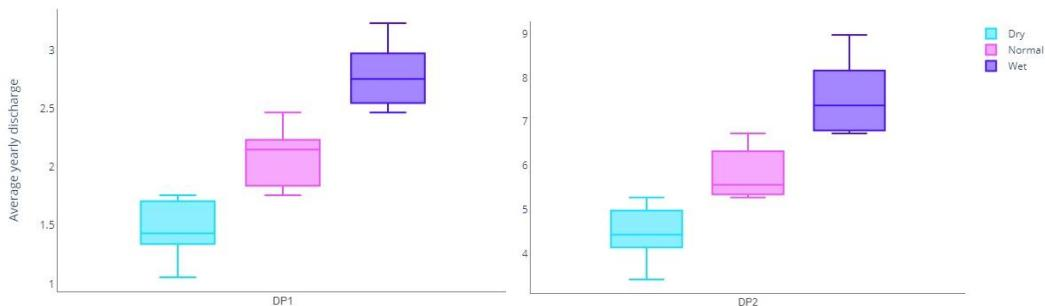
Figure 4 **Average yearly discharge values (in m<sup>3</sup>/s) for the considered scenarios (dry, normal and wet) for the two diversion points DP1 and DP2.** The upper and lower fences represent the max and min discharge values, the edges of the box represent the upper and lower quartiles, and the line inside the box is the median.
