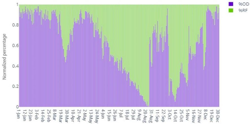
**Figure 8 Reference flow and optimized flow.** Comparison between the residual percentage of natural daily flow (green - %RF) remains in the river and the average daily discharge optimized for diversion (purple - %OD]). The diverted discharge is calculated as a daily average for all the 10 runs of the model. Presented results are for the DP1 under the dry scenario.
