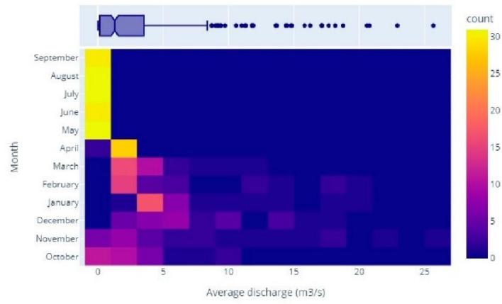
**Figure S11.** Heatmap showing the average optimized discharge (in m³/s) value (on the x-axis) for each month (on the y-axis) for the 2041 BAU\_CC scenario. On the right-hand side of the box a colour-based classification of the frequency of appearance of each value range; on top of the box a regular box-plot shows the yearly quartiles, extremes and outliers.
