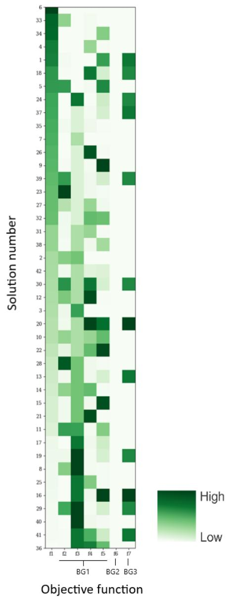
**Figure 6 Heat map of the objective functions.** Heatmap showing the sorted normalized objective functions scores [on the y-axis] for the e-flow requirements (BG1=Biological Group 1; BG2=Biological Group 2; BG3=Biological Group 3) in relation to the municipal water supply objective (f1) [on the x-axis]. Tiles hue indicates the score (dark green=high/best scores; light green=low/worst scores). Presented result is for run #1 for DP1, dry scenario.
