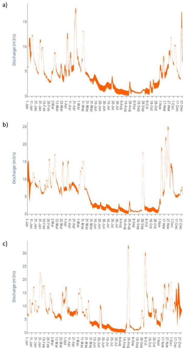
**Figure S7.** Flow series showing the magnitude of gap between the daily optimized diverted discharges in  $\text{m}^3/\text{s}$  with respect to the natural discharge. Greater thickness indicates the highest trade-off between the natural discharge and water for municipal use. **Results for DP2** under dry (a), normal (b) and wet (c) scenarios.
