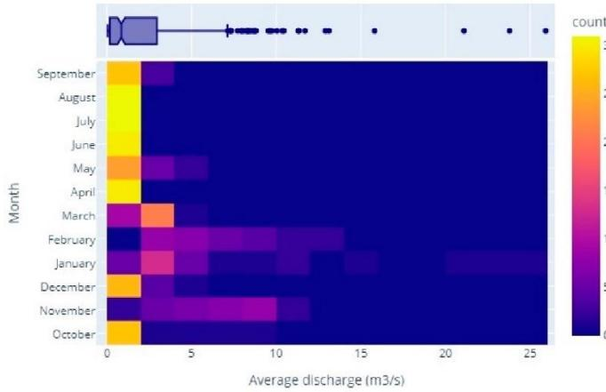
**Figure S13.** Heatmap showing the average optimized discharge (in m³/s) value (on the x-axis) for each month (on the y-axis) for the 2070 BAU\_CC scenario. On the right-hand side of the box a colour-based classification of the frequency of appearance of each value range; on top of the box a regular box-plot shows the yearly quartiles, extremes and outliers.
