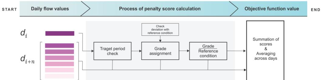
Figure 9 **General structure of the calculation process for the penalty score and objective function** ( $d_i$  and  $d_{i+n}$  indicate a day  $i$  of the year starting from January 1st).
