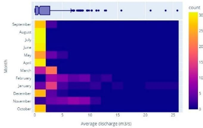
**Figure S12.** Heatmap showing the average optimized discharge (in m³/s) value (on the x-axis) for each month (on the y-axis) for the 2070 BGIN\_CC scenario. On the right-hand side of the box a colour-based classification of the frequency of appearance of each value range; on top of the box a regular box-plot shows the yearly quartiles, extremes and outliers.
