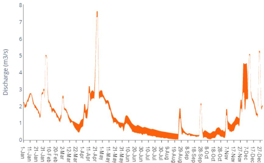
**Figure 9 Gap between optimized and natural flow.** Flow series showing the magnitude of gap between the daily optimized diverted discharges with respect to the natural discharge for the DP1 under the dry scenario. Greater thickness indicates the highest trade-off between the natural discharge and water for municipal use.
