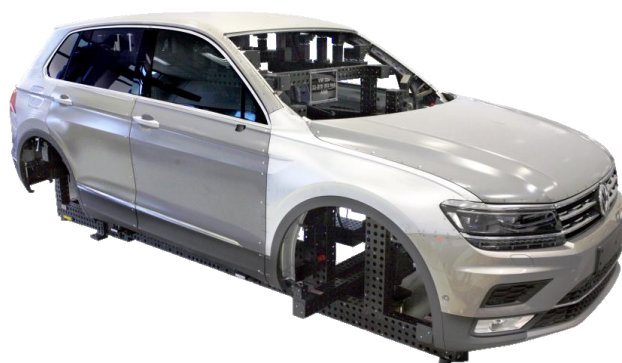
Figure 3: Exterior parts of Volkswagen Tiguan mounted on the corresponding Meisterbock
