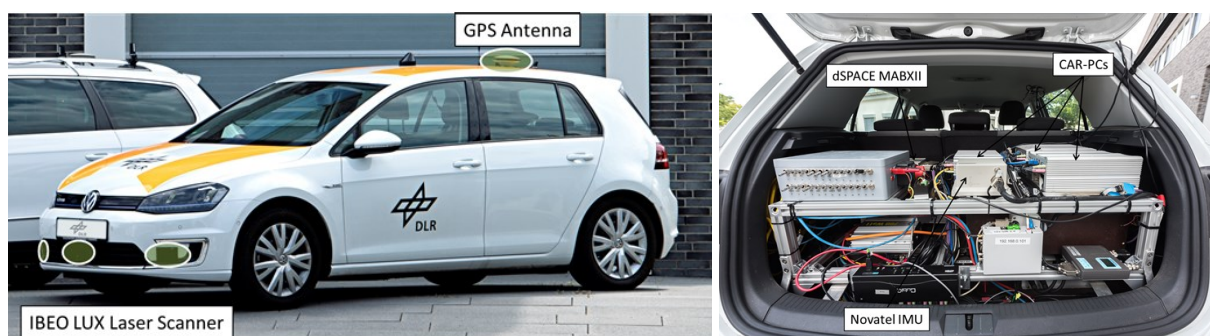
Figure 10: Left: Sensors of FASCarE. Right: Trunk installments of FASCarE
