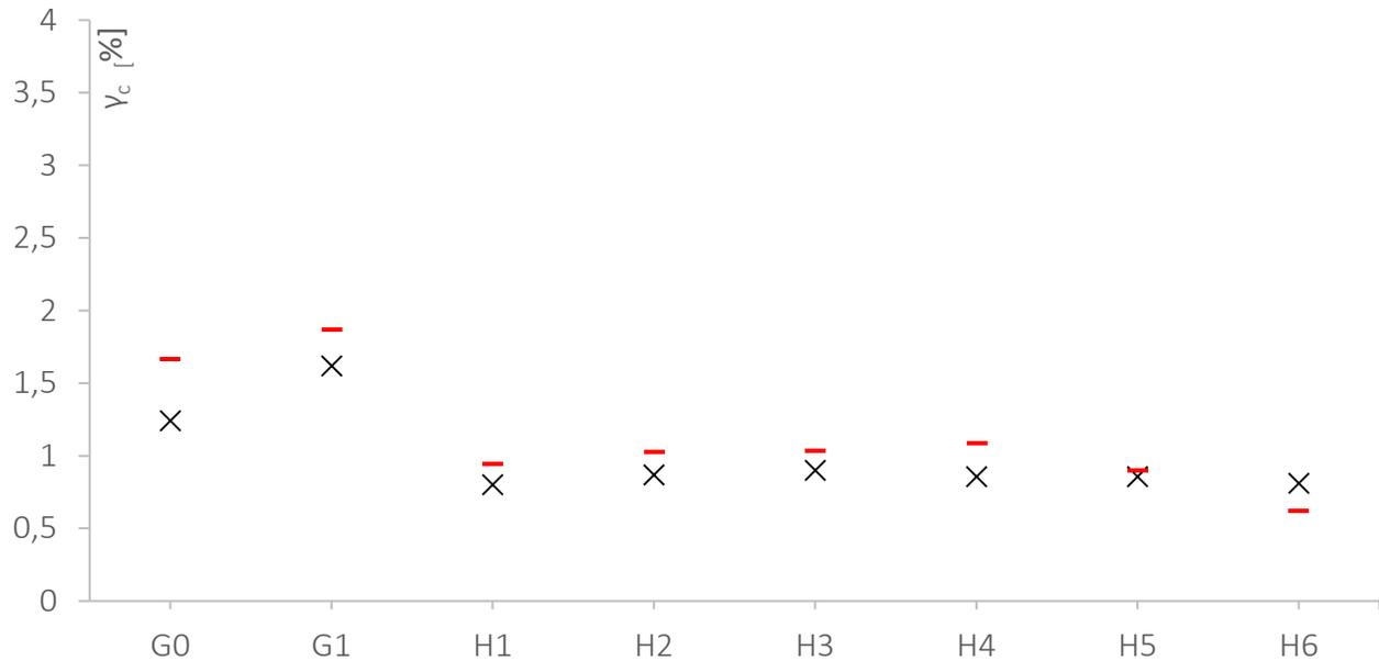
Figure 3.31. Critical strain  $\gamma_c$  of the creams G0 and H1 to H6 one day after the preparation (X) and after 6 months storage (-) at RT.  $\gamma_c$  is expressed as a percent of the strain range during the strain test ( $\gamma$  from 0 to 5) and taken at  $\tan\delta = 1$ .
