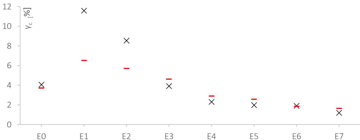
Figure 3.7. Critical strain  $\gamma_c$  of the creams E0 to E7 one day (X) and 6 months (-) after preparation (storage at RT).  $\gamma_c$  is expressed as a percent of the total strain range during the amplitude test ( $\gamma$  from 0 to 5) and taken at  $\tan\delta = 1$ ,  $\omega = 1.6 \text{ Hz}$ .
