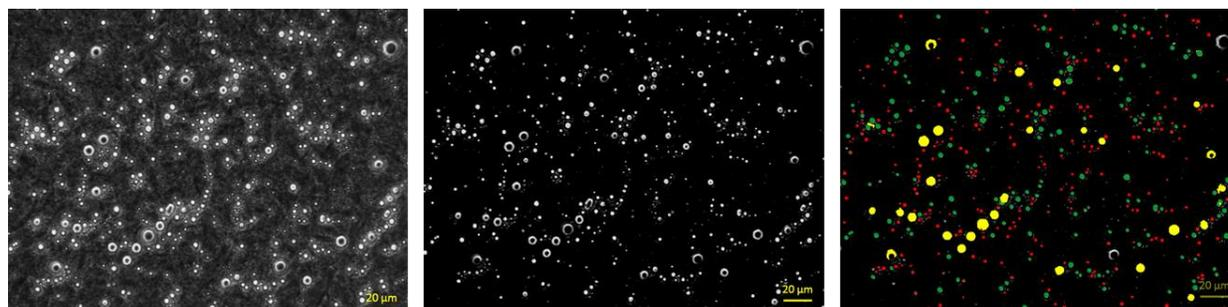
Figure 3.26. Description of the automatic particle recognition process for particle size distribution calculation in the nonionic creams using the software ZEN (image analysis module Blue) from Zeiss. Left and middle photomicrographs: PC pictures of the cream H3 before and after isolation of the “objects” (i.e. isolation of the particles from the background). Right: Automatic particle recognition. The yellow dots show
