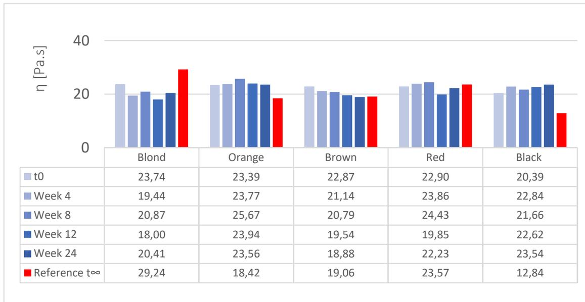
Appendix 7.7.iii. Viscosity of the nonionic creams and the reference ionic creams (shades: black, brown, orange, red, and blond) from t0 to month 6 storage at RT. The viscosity  $\eta$  is measured at  $\dot{\gamma} = 7,2 \text{ s}^{-1}$  at 20°C.
