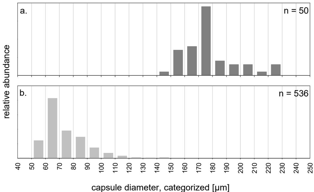
**Figure 4-7:** *Relative abundance of capsules within size categories of the capsule diameter depending on two different capillary diameters for the functional phase (ACPM) for the same flow rate. Inner capillary diameter: a. 130  $\mu\text{m}$ , b. 65  $\mu\text{m}$ . n = sample size. Encapsulation parameters: flow rate ACPM = 0.2  $\mu\text{L min}^{-1}$ , flow velocity oil = 2 m  $\text{min}^{-1}$ .*
