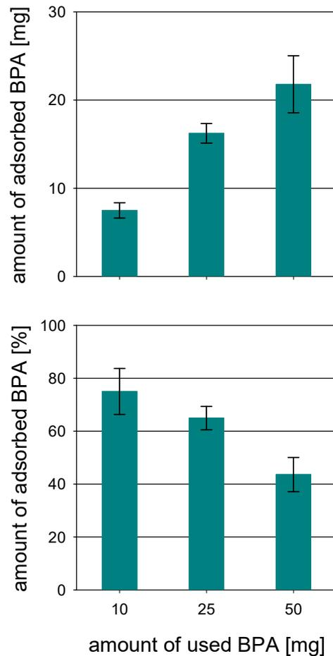
**Figure 3-2:** Adsorption of BPA on granulated activated carbon out of the aqueous phase.
