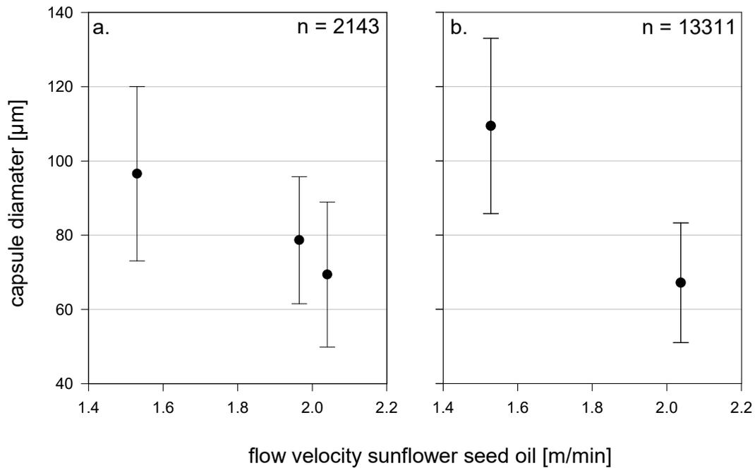
**Figure 4-9:** ‘Mean capsule diameter’ capsules depending on different flow velocities of the continuous phase (sunflower seed oil). Flow-rate for the functional phase (ACPM) = a.  $0.2 \mu\text{L min}^{-1}$  and b.  $0.1 \mu\text{L min}^{-1}$ .  $n$  = sample size.
