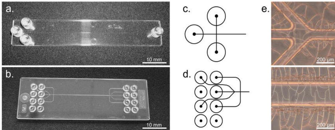
**Figure 4-3:** Tested commercial microfluidic chips (microfluidic ChipShop GmbH, Jena, Germany): a. Cross-shaped channel chip (PMMA) with channel diameters of 50  $\mu\text{m}$  and b. Droplet generator chip (PC) with channel diameters of 70  $\mu\text{m}$ . c. and d. Schematic drawing of the geometry of the respective microfluidic application for droplet generation. e. Micro cracks, which arise through excessive use.
