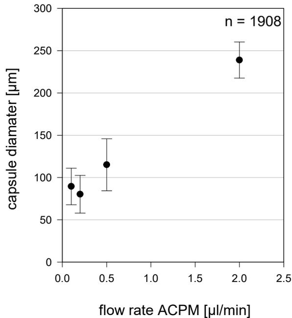
**Figure 4-8:** *'Mean capsule diameter' capsules depending on different flow rates of the functional phase (ACPM). Flow velocity for the continuous phase (sunflower seed oil) = 1 m min<sup>-1</sup>. n = sample size.*
