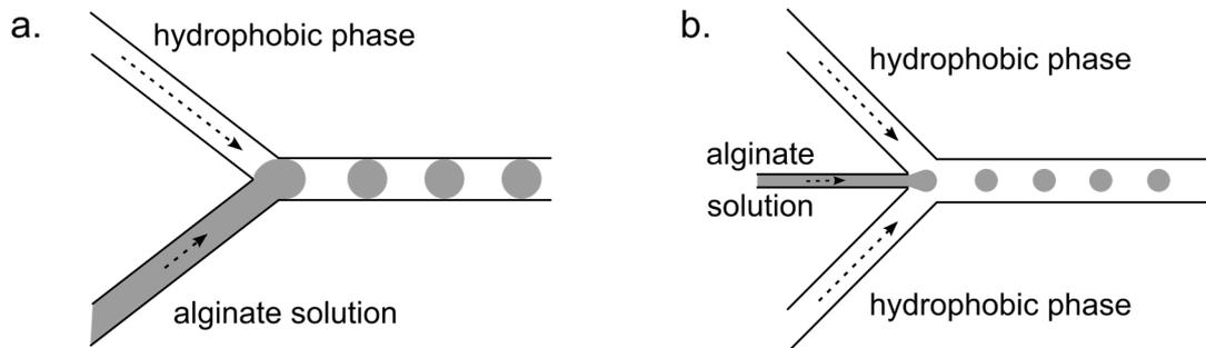
**Figure 4-2:** Common schematic geometries of microfluidic devices for the production of alginate microcapsules: a. 'Y' junction squeezing channel and b. flow focussing channel.
