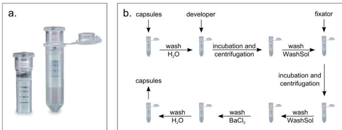
**Figure 4-10:** *Microautoradiography with microencapsulated cells. a. Centrifugal filter units with vertical polyethersulfone membranes. b. Applied sequence of different washing, development and fixation steps.*
