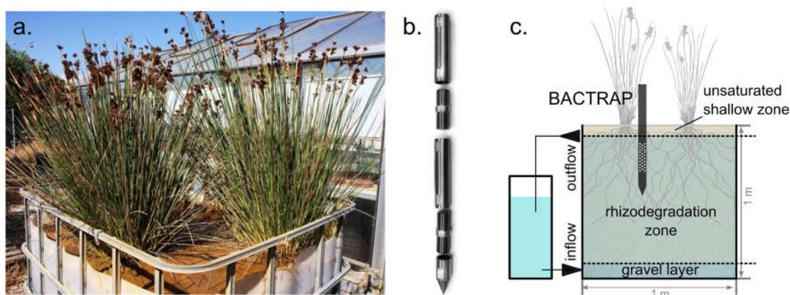
**Figure 3-1:** *Experimental setup of the SIP-BACTRAP test in a Shallow Aquifer Rhizodegradation pilot-plant in Chania. a. Photography of the investigated system. b. Direct-push BACTRAP (threefold segmented for parallel exposition of blank,  $^{12}\text{C}$  and  $^{13}\text{C}$ ) for insertion into overgrown rhizosphere. c. Schematic drawing of the rhizodegradation system and BACTRAP placement.*
