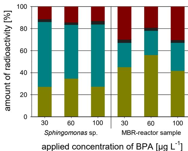
**Figure 3-5:** Fate of BPA in the mineralisation experiment. The distribution of <sup>14</sup>C-label in the NaOH reservoir (■), aqueous supernatant of the cultures (■), the biomass (■) and the ethyl acetate washing extract (■) for *Sphingomonas* sp. strain TTNP3 and the sample of the MBR reactor was measured.
