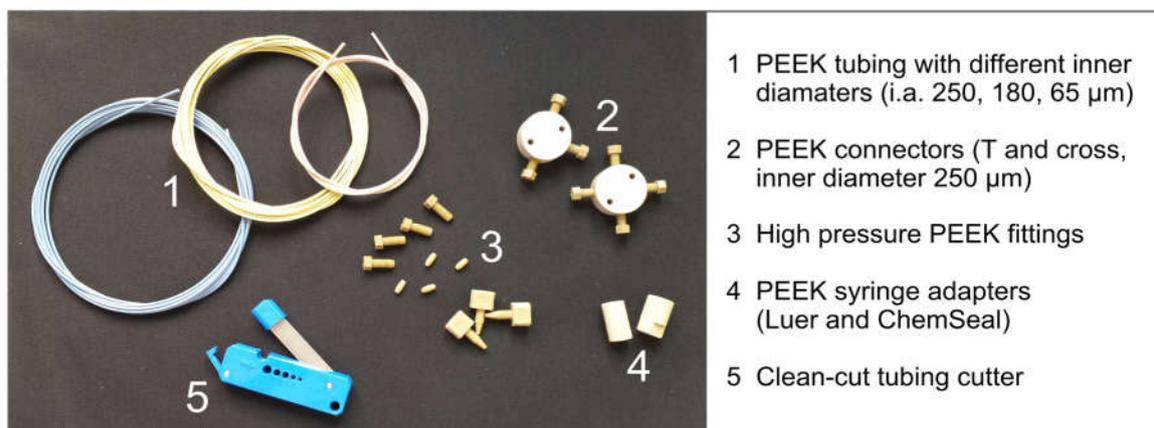
**Figure 4-4:** Set of PEEK accessories used for microencapsulation of cells into alginate matrix.
