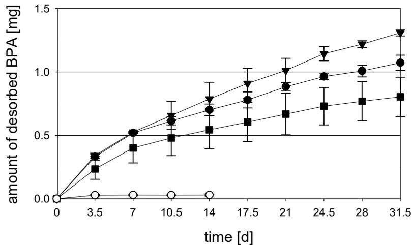
**Figure 3-3:** Desorption of BPA from granulated activated carbon into the aqueous phase. Shown are the desorption kinetics of the carrier material, loaded with 50 mg (unfiltered supernatant ●; filtered ○), 25 mg (unfiltered ▼) and 10 mg (unfiltered ■) substrate.
