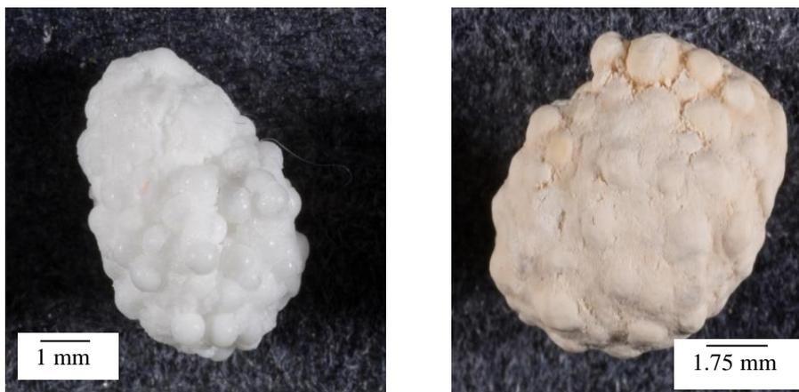
Figure 44: Irregularly shaped pellets produced at processing time of 15 min., a binder content of 0.053 g/g , a) Rotational speed 0.17 m/s and alumina primary particles with  $d_{50,3} = 1.0$  mm, b) Rotational speed 0.74 m/s and zeolite primary particles with  $d_{50,3} = 1.75$  mm.
