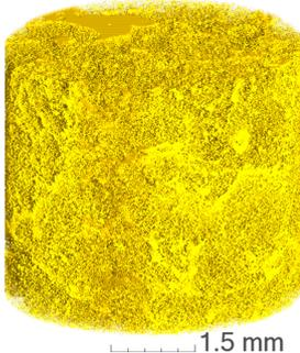
FIGURE 3.2: Pore system on the same 7 mm wide subvolume of a 10 cm  $\varnothing$  sample and the corresponding 3 cm  $\varnothing$  and 0.7 cm  $\varnothing$  subsamples at the identical position reveal the relationship between sample size and resolution.
