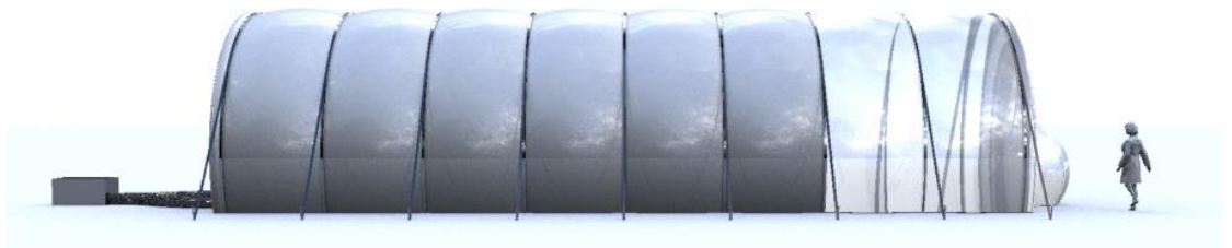
Figure 17 - Isometric view, Cylindrical Hangar Structure.
