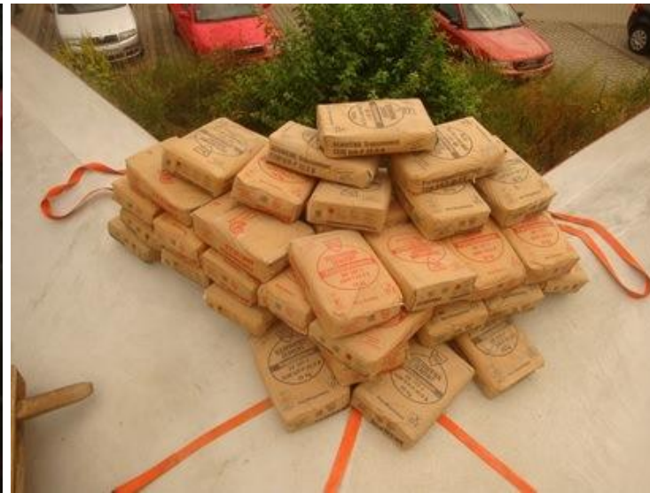
Load Test II-2 – 50 bags ~ 1,250 kg.
