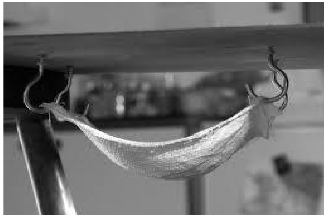
Figure 3.43 – Heinz Isler models of shells based upon hardened hanging clothes and inverted shells.
