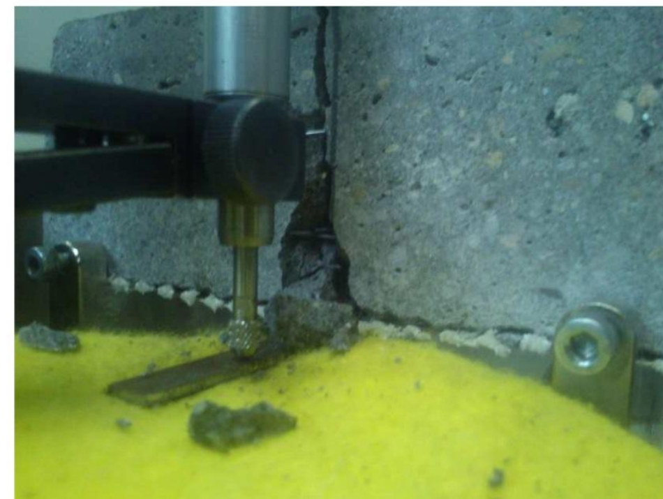
Figure 5.35 – Experimental 3-Point set-up of Flexural Testing of Concrete samples of IMS Membrane-Concrete Shell Prototype.
