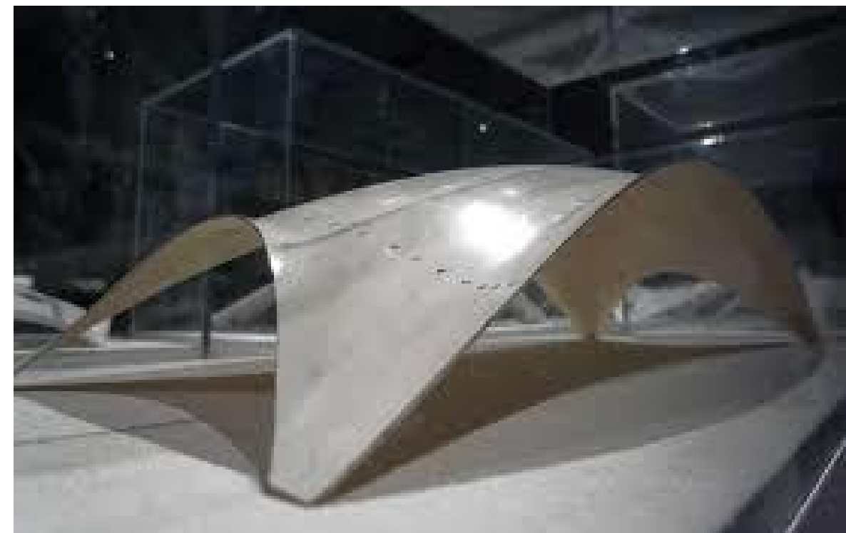
Figure 3.43 – Heinz Isler models of shells based upon hardened hanging clothes and inverted shells.
