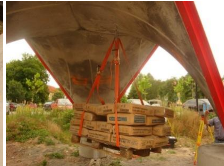
Load Test III-1 – 27 bags ~ 675 kg.
