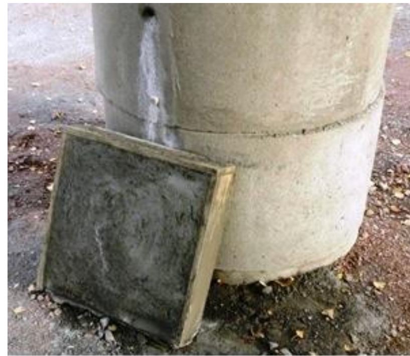
45x45 cm. Square Shotcrete Specimen - "Spritzkissen"
