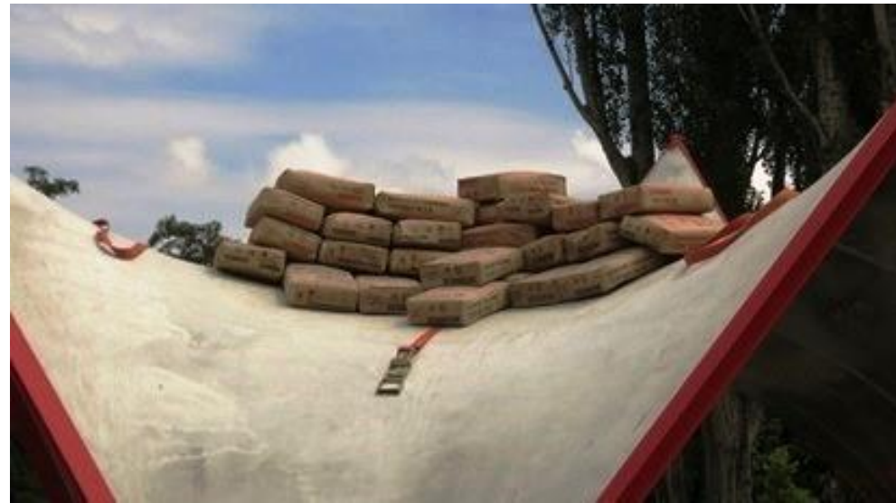
Load Test II-1 – 30 bags ~ 750 kg.
