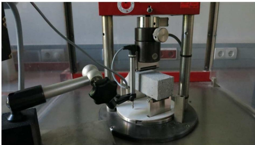
Testing rig (3 point flexural testing) with external displacement transducer
