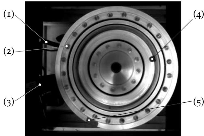
Figure 6.19.: Single frame of the 240 fps test bench recording at a momentary rotor speed of 1200 rpm. (1) Encoder stand (2) unbalance mass (3) laser triangulation sensor (4) ball (5) visual zero marking.
