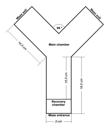
Figure 1. Schematic diagram of the Y-maze apparatus for the choice experiments (reconstruction, following Bruce et al. 2001).
