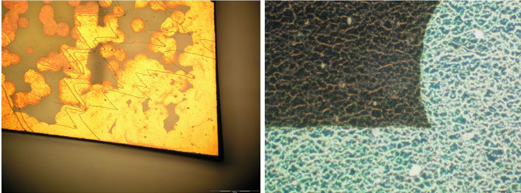
Figure 3.23: Microscope photographs of sample between two removal baths (left) in bright field and (right) the in dark field observed chemical removal frontier.
