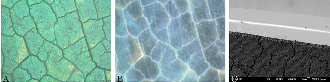
Figure 3.25: BF (A) and DF (B) microscope views of a PMMA opal sample: the cracks become visible in DF, but as well the very fine structures of small scratches and defects can be seen; DF illumination uses scattered light to identify inhomogeneities (Olympus BX51, M=100 objective, NA=0.9). (C) shows a thin-film opal on silicon under SEM with pronounced drying cracks.
