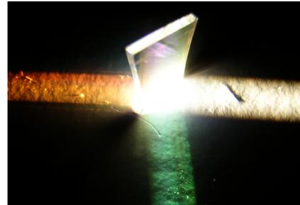
Figure 3.31: inverted opal beamsplitter on glass.
