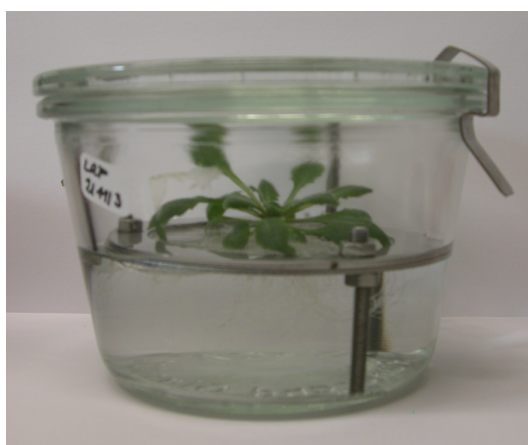
Figure 55: Hydroponic culture system for controlled growth conditions and easy root harvest
