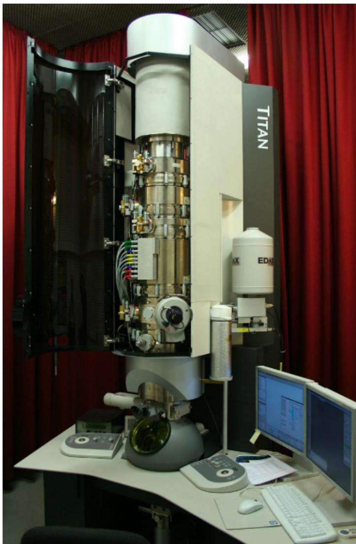
Fig. 3.7: LTEM system (TITAN 80-300 from FEI)
