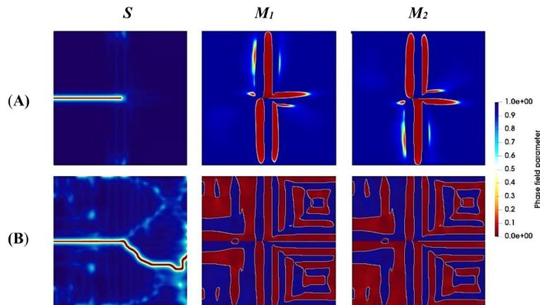
Fig. 3: Evolution of the crack field (S) and martensitic variants (M1, M2) by considering two variants of martensite. Rows (A) and (B) correspond to times 4 μs, and 45 μs.
