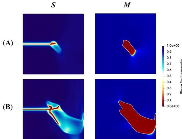
Fig. 2: Evolution of the crack field (S) and martensitic variant (M) by considering one variant of martensite. Rows (A) and (B) correspond to times 6 μs, and 36 μs.
