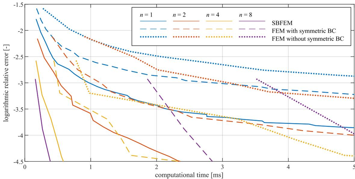
**Fig. 1:** Comparison of the error and the computational time of the SBFEM (solid lines) and two FEM models (dashed and dotted lines) for different node numbers (the node numbers vary along the line paths) and for shape functions of different polynomial degrees  $n$  (colors).
