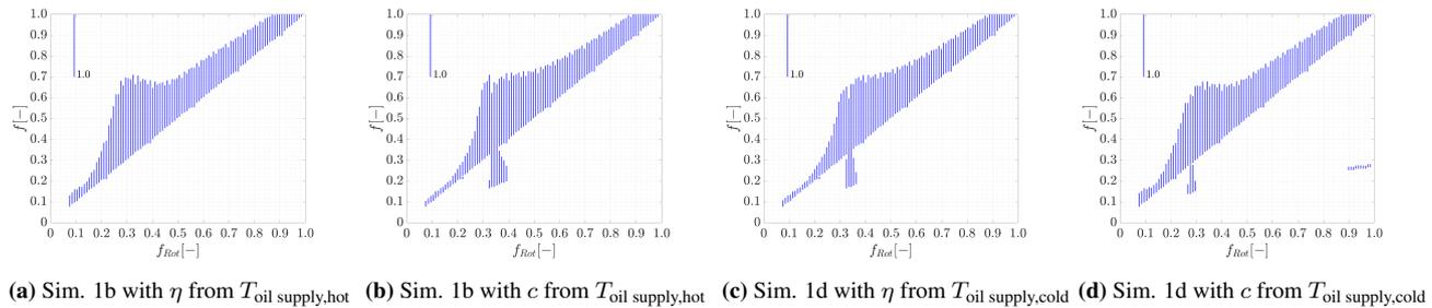
**Fig. 2:** Influences of thermally dependent viscosity  $\eta$  and bearing clearance  $c$  at  $T_{oil\ supply,cold}$  (Figs. 2a, 2b) and  $T_{oil\ supply,hot}$  (Figs. 2c, 2d)
