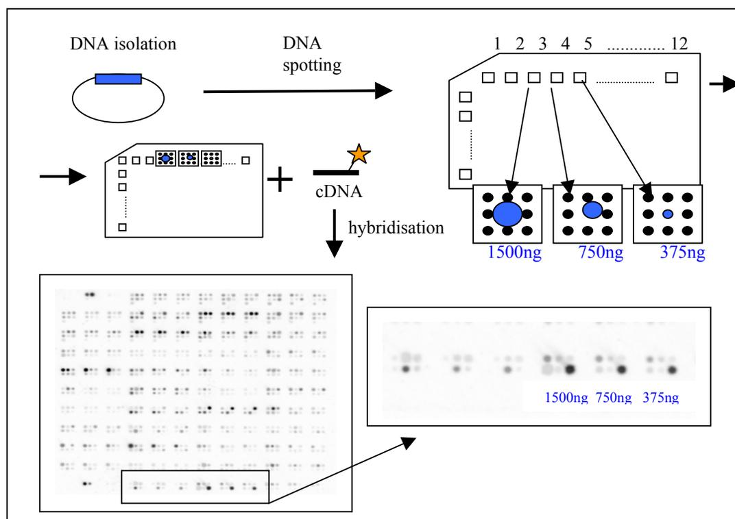
Fig. 5.2 The schematic representation of macroarray used in this study. Purified DNA was spotted on a nylon membrane in a pattern 3x3. DNA, each corresponding to a particular gene, was applied in concentrations 1500 ng, 750 ng and 375 ng in neighbouring patterns. Messenger RNA purified from total RNA via dynabeads was reverse transcribed and cDNA labelled with  $[\alpha\text{-}^{33}\text{P}]\text{dCTP}$ . For more detailed description and hybridisation conditions see Chapter 7.
